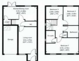
GROUND FLOOR 1ST FLOOR
